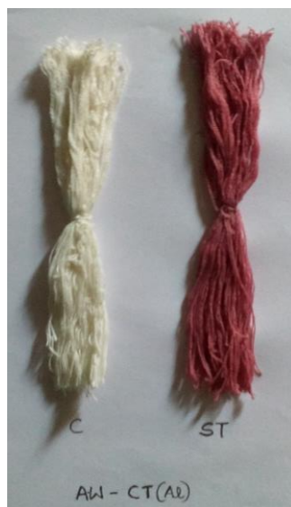
Figure11: Dyeing of cotton yarn with A.wilkesiana (70°C,pH6,45min,ML-1:40)
