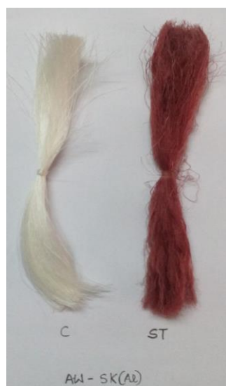
Figure 12: Dyeing of silk yarn with A.wilkesiana (60°C,pH5,1hr,ML-1:40)
