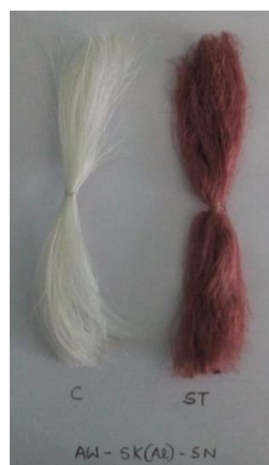
Figure14: Dyeing of silk yarn with A. wilkesiana in sonicator (60°C,pH5,15min,ML-1:40)
