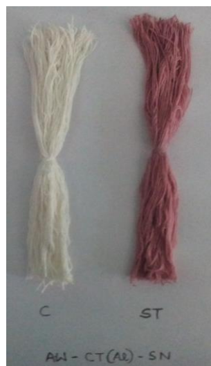
Figure13: Dyeing of cotton yarn with A. wilkesiana in sonicator (60°C,pH6,15min,ML-1:40)
